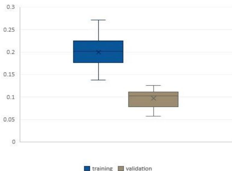
*Figure 5.14 Variability of the model predictive capacity (explained variance values from 100 x bootstrap) in training and validation.*
